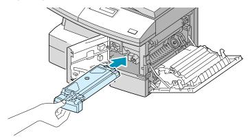
7 Turn the cartridge locking lever downwards until it locks into place.
